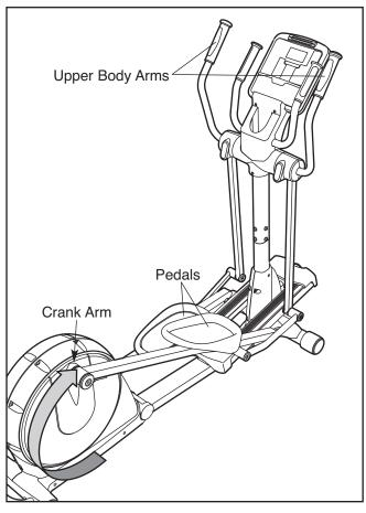
Note: The crank arms can turn in either direction. It is recommended that you turn the crank arms in the direction shown by the arrow; however, for variety you can turn the crank arms in the opposite direction.
